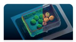
RGB-D solution — If the depth values of the Basler ToF Camera are combined with color values recorded by a separate RGB camera, point clouds can be displayed in the colors that are actually present. This can help to compensate for missing depth information, perform additional classifications based on object color, or facilitate scene understanding.
