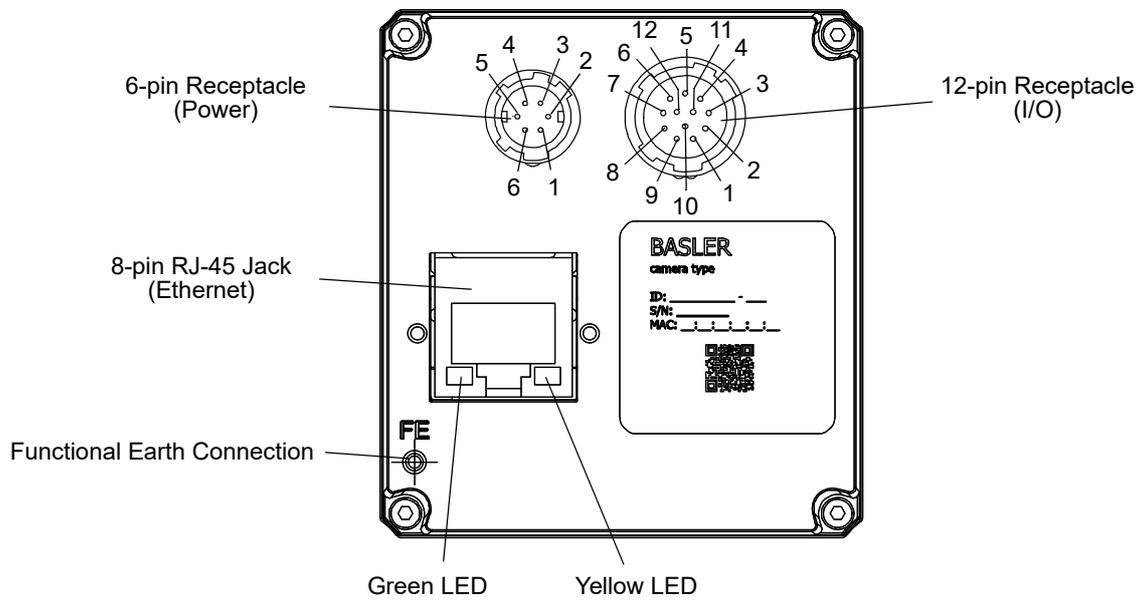
Fig. 16: Camera Connectors , LEDs, FE Connection, and Pin Numbering for the 6-pin and 12-pin Receptacles
