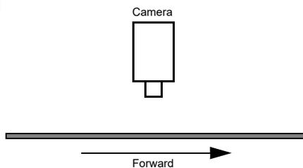
The conveyor resumes forward motion and the shaft encoder module begins generating forward ticks. The reverse counter will decrement by 1 for each forward tick. While the reverse counter is decrementing, the output of trigger signals from the module is suppressed. When the reverse counter decrements to 0, decrementing stops and suppression of the trigger signals stops. The module will begin outputting a trigger signal for each forward tick received.
