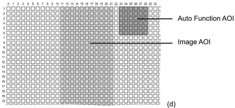
Fig. 56: Various Degrees of Overlap Between the Auto Function AOI and the Image AOI
