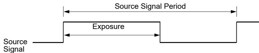
Fig. 28: Trigger Width Exposure with RisingEdge Line Start Triggering
