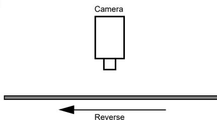
The conveyor resumes reverse motion and the shaft encoder module begins generating reverse ticks.
