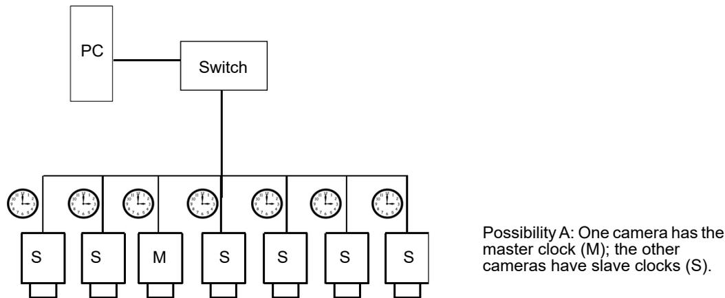
Fig. 60: PTP-capable Cameras Using the Same System Time
