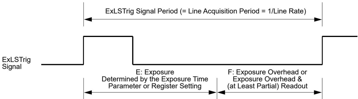
Fig. 44: Relation of the ExLSTrig Signal Period and Periods E and F for Regular Line Acquisition in Timed Exposure Mode
