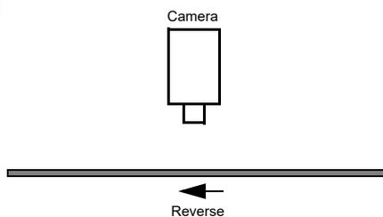
The conveyor jitters and moves briefly in reverse. During this reverse movement, the shaft encoder generates 5 reverse ticks. The reverse counter will increment by 1 for each reverse tick and when the reverse motion stops, the reverse counter count will be 5. While the reverse counter is incrementing, the output of trigger signals from the module is suppressed.
