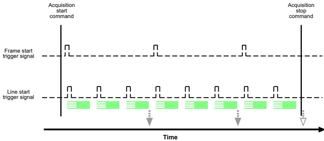
Fig. 31: Use Case 2 - Continuous Frame Mode with Acquisition Start, Frame Start and Line Start Triggering Set to Off
