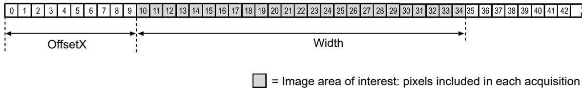
Fig. 27: Pixels Used for Each Line Acquisition
