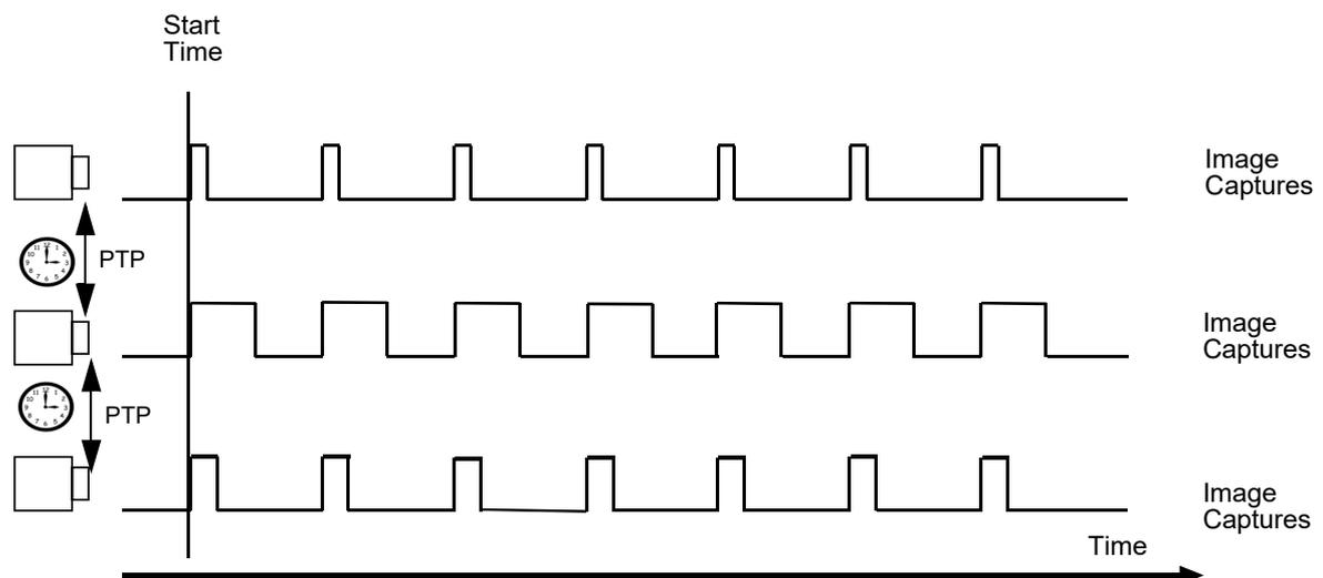
Fig. 66: **Example D:** Same Start Time and Same SyncFreeRunTriggerRateAbs but Different Exposure Times
