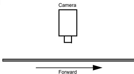
The conveyor is moving forward and the encoder is generating forward ticks. Whenever the module receives a forward tick, it outputs a trigger signal. The reverse counter is at 0.
