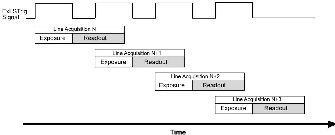
Fig. 40: Overlapped Exposure and Readout
