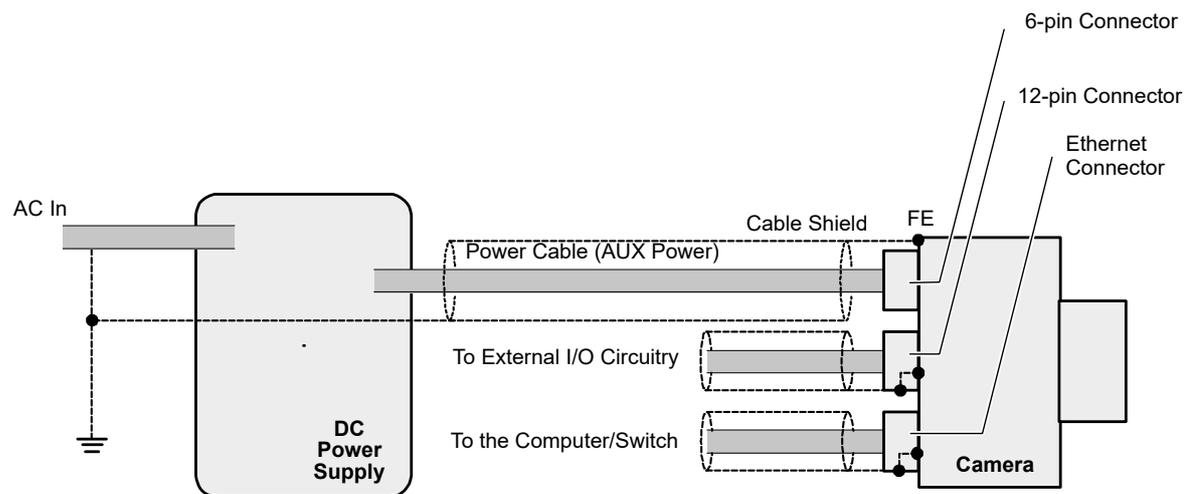
Fig. 17: Grounding Scheme for Power Supply, Power Cable, and Camera
