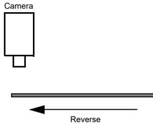
The conveyor begins moving in reverse and the shaft encoder starts generating reverse ticks.
