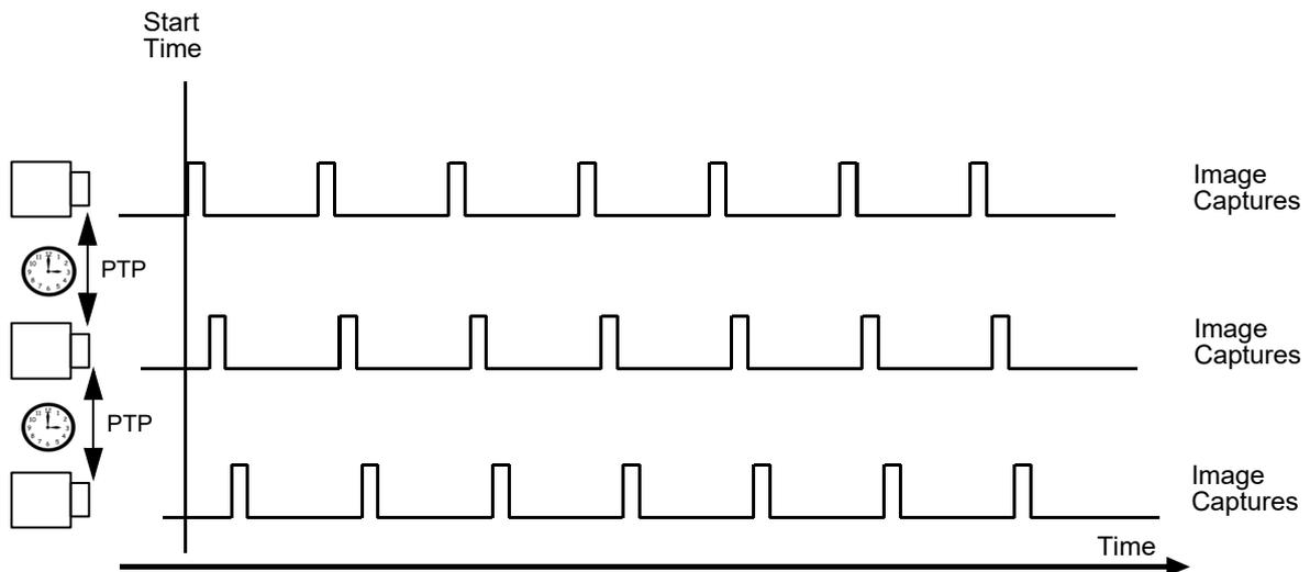
Fig. 65: **Example C:** Same SyncFreeRunTriggerRateAbs but in Chronological Sequence
