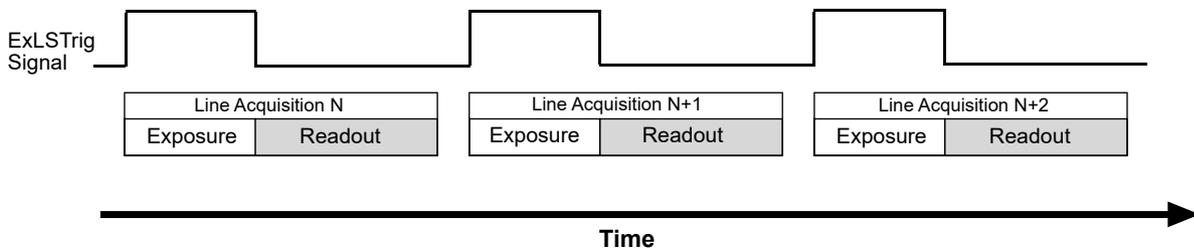
Fig. 39: Non-overlapped Exposure and Readout
