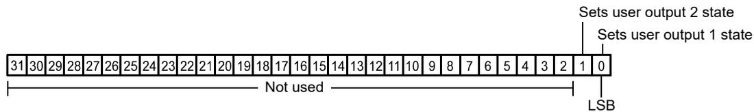
Fig. 25: User Output Value All Parameter Bits
