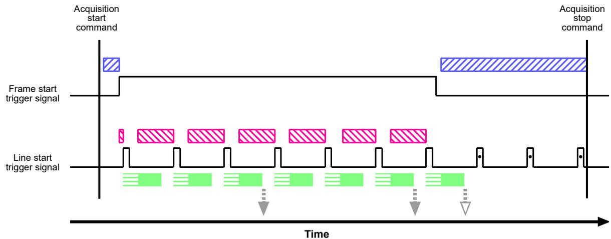
Fig. 35: Use Case 6 - Continuous Frame Mode with Acquisition Start Triggering Set to Off, Frame Start and Line Start Triggering Set to On, and TriggerPartialClosingFrame set to True
