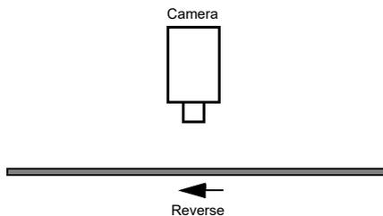
The conveyor jitters and moves briefly in reverse. During this reverse movement, the shaft encoder generates 5 reverse ticks. The reverse counter will increment by 1 for each reverse tick and when the reverse motion stops, the reverse counter count will be 5.
