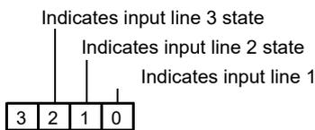
Fig. 70: Input Status At Line Trigger Parameter Bits
