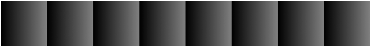
Fig. 83: Test Image Eight for 8 bit Output Modes, Generated with a Raw or Enhanced Raw Line Acquisition Mode on a Camera with 4096 Pixels Per Line
