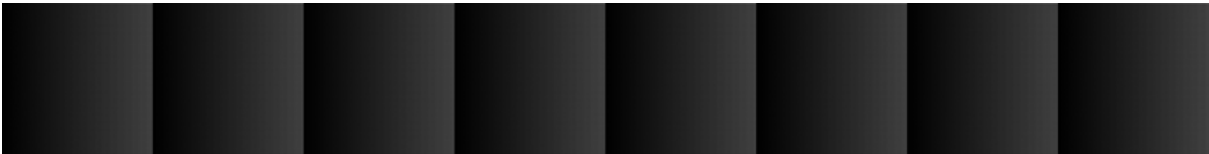
Fig. 80: Test Image Seven for 8 bit Output Modes Generated with a Raw or Enhanced Raw Line Acquisition Mode (Raw - Line A First and Enhanced Raw - Line A First as an Example) on a Camera with 4096 Pixels Per Line
