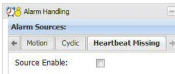
**Source Enable** - Check the **Source Enable** box on the **Heartbeat Missing** tab to enable the heartbeat missing alarm source for declaring an alarm condition when the heartbeat timeout expires.
