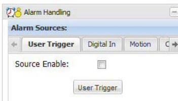
**Source Enable** - Check the **Source Enable** box on the **User Trigger** tab to enable the user trigger as a source for declaring an alarm condition.
