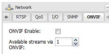
**ONVIF Enable** - Check the **ONVIF Enable** box to enable the camera for ONVIF support. By default, the ONVIF support is disabled.
