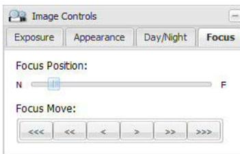
**Focus Position** - Indicates the relative focus position between near (N) and far (F).
