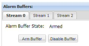
**Alarm Buffer State** - Indicates the current state of the alarm buffer for stream 0.
